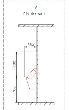
Water piping — inclined for discharging (won't be fully discharged)
